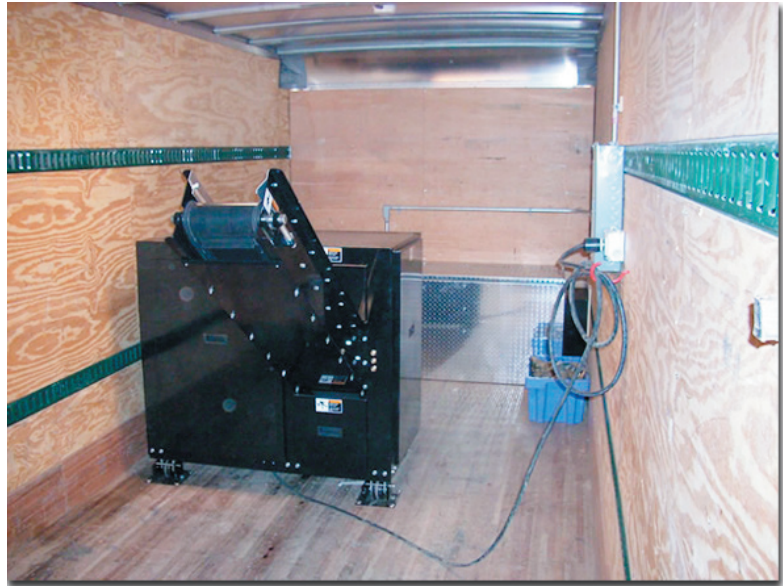
Series 2 Hard Drive Shredder Installed
